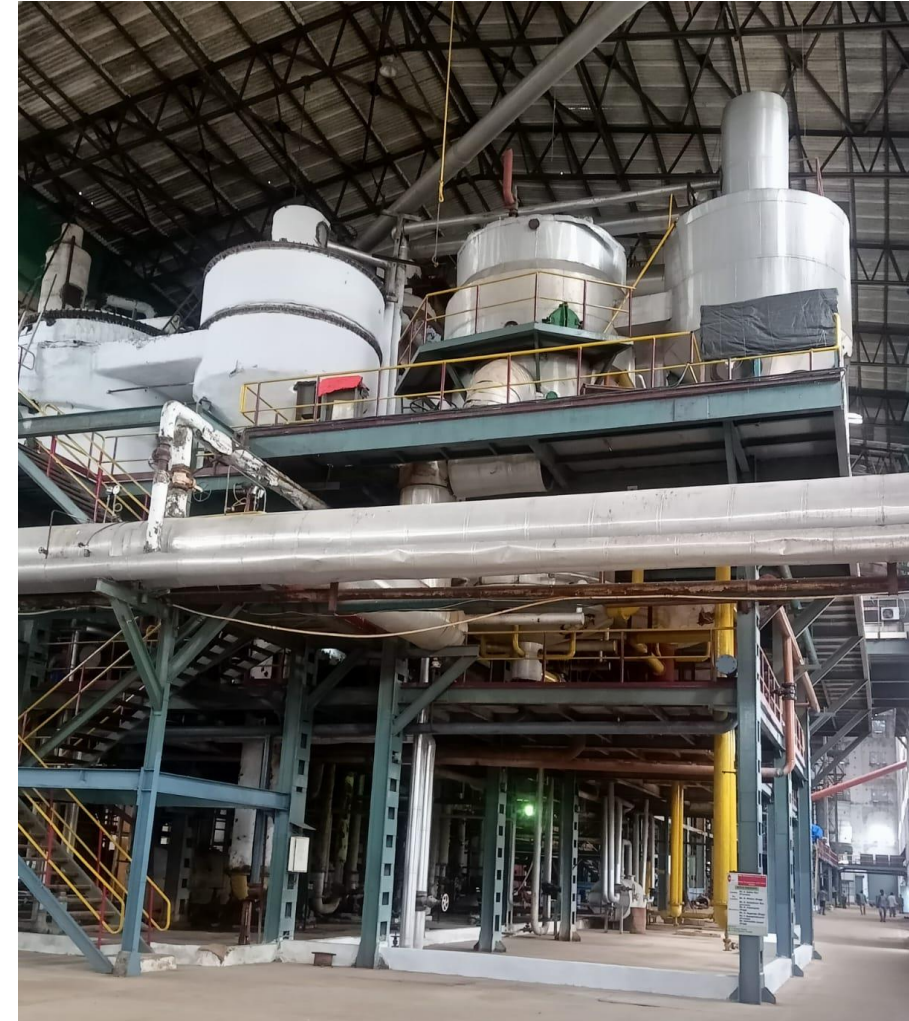
Picture 2: (a) Mill house: the cane is crushed to extract juice and (b) Boiling house: impurities are removed from sugarcane juice
