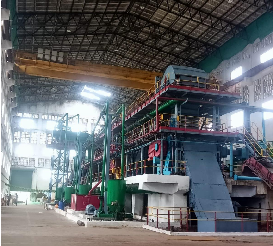
Picture 2: (a) Mill house: the cane is crushed to extract juice and (b) Boiling house: impurities are removed from sugarcane juice
